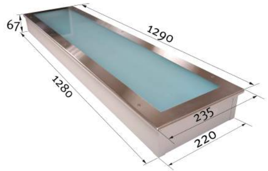
CLUX122: 1.280 x 220 x 67 (mm). Fluorescentes: 2 x 54W - T 5 - 220V.
