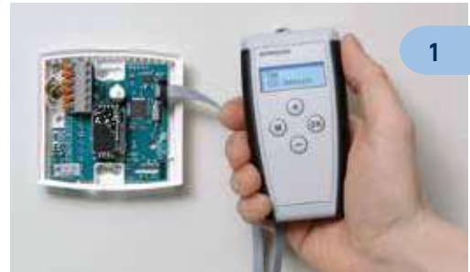
2 Easy tuning of the duct sensor's temperature measurement
