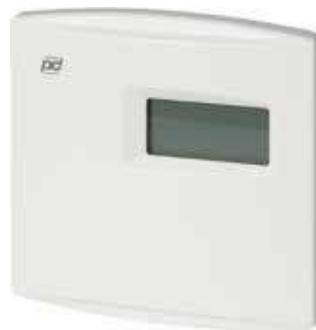
*TEHR LL (2-wire, 4...20 mA) and TEHR LU (3-wire, 0...10 V) are temperature transmitters for dry room spaces. The output range is selectable. TEHR-M output is available via Modbus and as a 0...10 V signal.*
